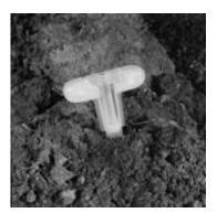
With the plunger seated in the handle, push the TerraCore into freshly exposed soil until the sample chamber is filled. A filled chamber will contain approximately 5 grams of soil.
